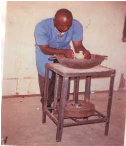
Plate 1: Final construction of a stand and kick-wheel
